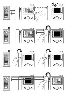
When an active call is open, select the internal receiver to which the call is to be transferred.
